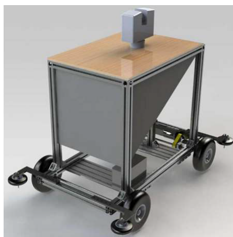
Figure 2. CAD of the carrying system for the laser scanner designed in [1]
